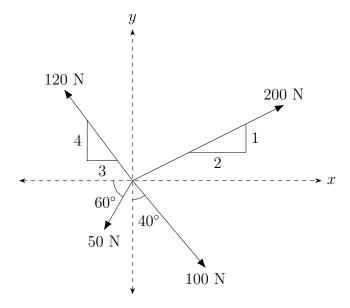
Let R be the resultant force with  $R_x$  being the horizontal component and  $R_y$  being the vertical component,
